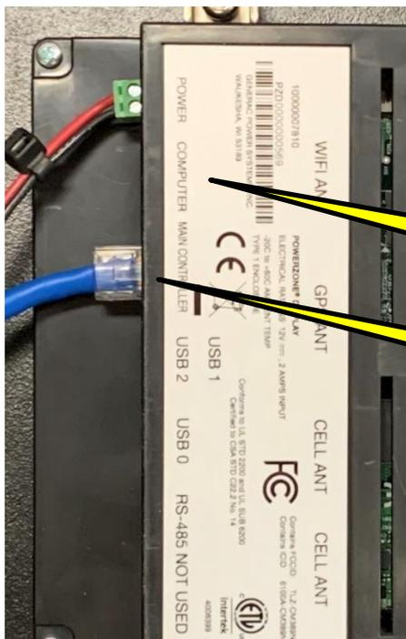
The OMNI CAT5 cable goes into the top RJ45 connector, initially labeled "COMPUTER"
