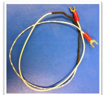
20K OHM Resistor Wire
