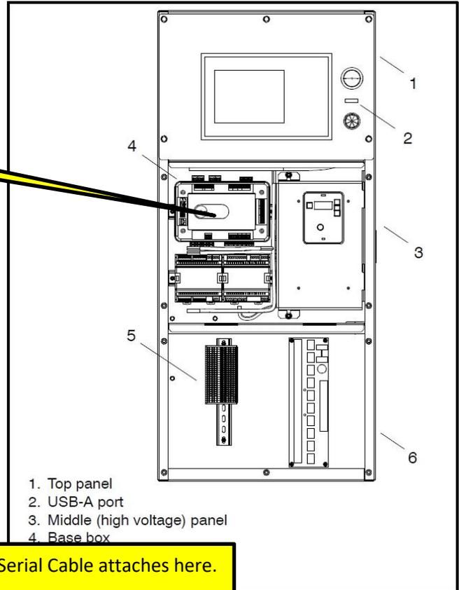
OMNI RS-232 Serial Cable attaches here.
